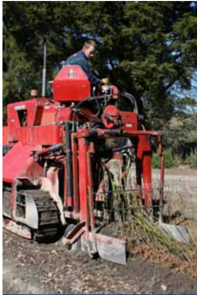
Appletons' custom-made mechanical lifter ensures easy, damage-free lifting of the young trees
