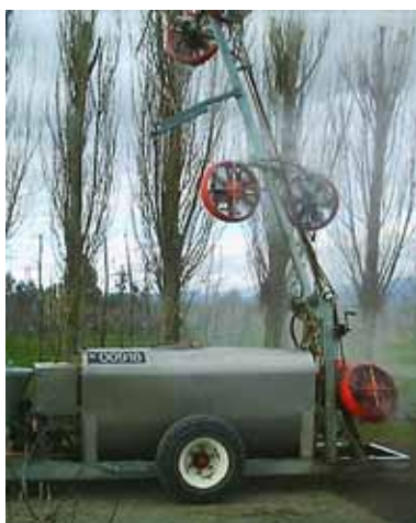
One of the early Quantum Mist sprayers built by New Zealander George Eady, original developer of the Quantum Mist sprayer technology
